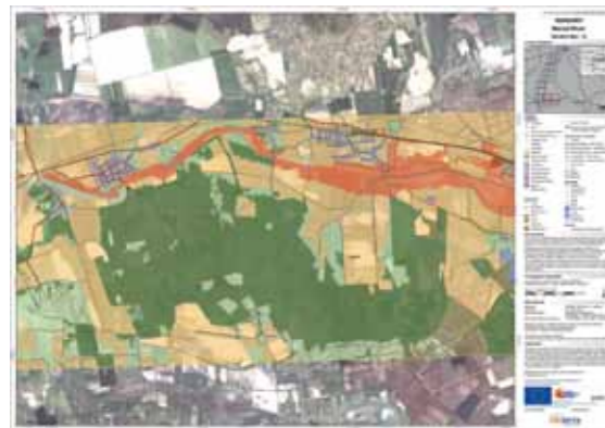
Detailed Damage Assessment Map - Detail Downstream of collapsed tailings reservoir near Kolontár, Hungary, in 2010 (1: 15,000) [Source: Astrium (SAFER)]
